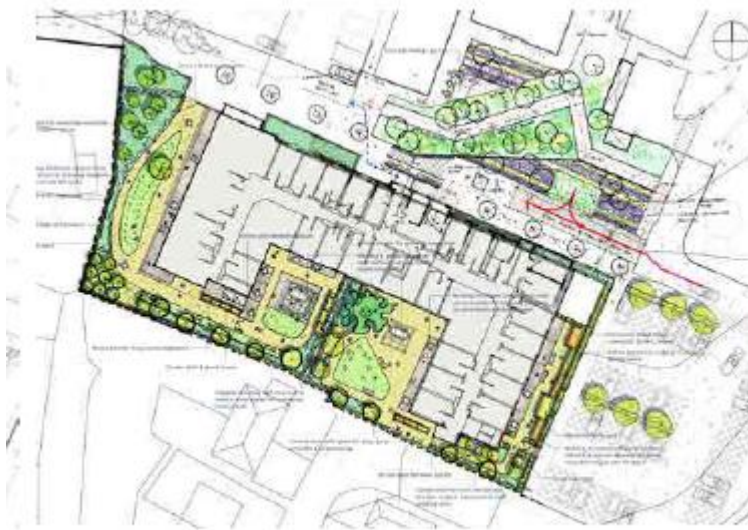
2. Developed proposal allowing rationalisation of private garden space and allowance for vehicle turning area in front of main entrance
